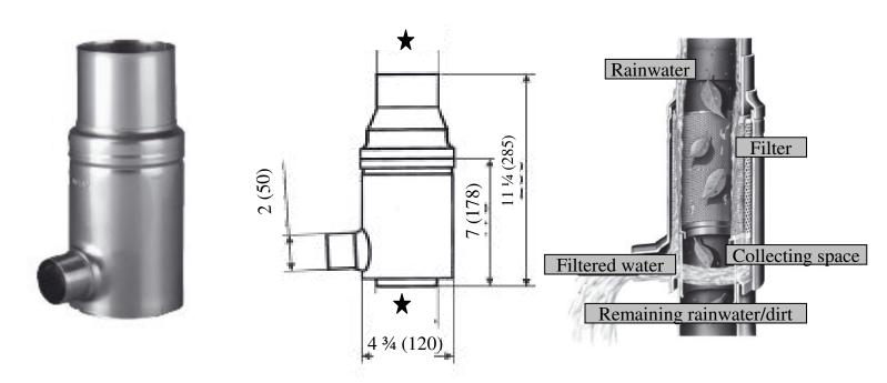
The garden filter is available in a variety of sizes to fit metal downspouts with internal diameters of 3 (76),  $3\frac{1}{8}$  (80),  $3\frac{1}{2}$  (87) and 4 (100) or plastic downspouts with internal diameters of  $2\frac{3}{4}$  (70, external diameter  $2\frac{15}{16}$  (75)) or 4 (100, external diameter  $4\frac{1}{3}$  (110)).
