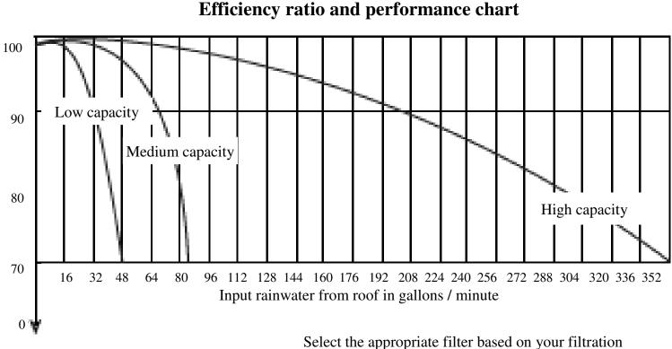
Select the appropriate filter based on your filtration needs and design flow rate.
