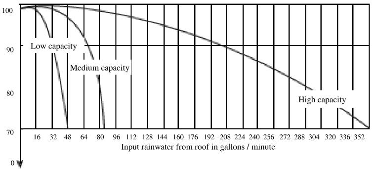
Select the appropriate filter based on your filtration needs and design flow rate.
