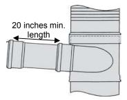
Connect 6" thin wall sewer and drain (S&D) piping\* to the inlet of the filter. Plumbing lubrication may be necessary to insert the S&D pipe into the intake gasket of the filter. Ensure there is at least 20 inches of flat pipe to calm water before entering the filter. Failure to do so will decrease filter efficiency. Wisy filters are made in Germany, thus the filter connections are in millimeters and require a ferncoat fitting (not included, but available from RMS) to make the
